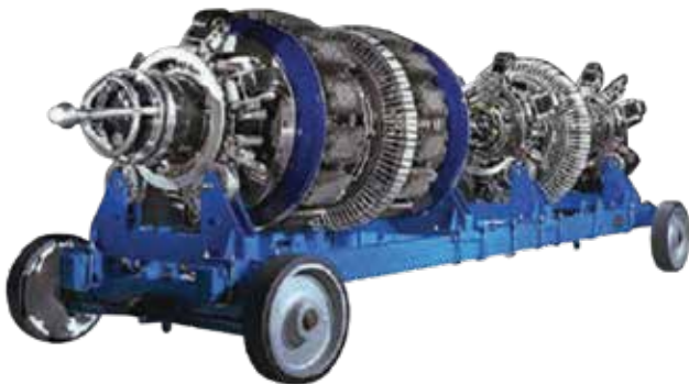
Smart Pig: An internal inspection tool
